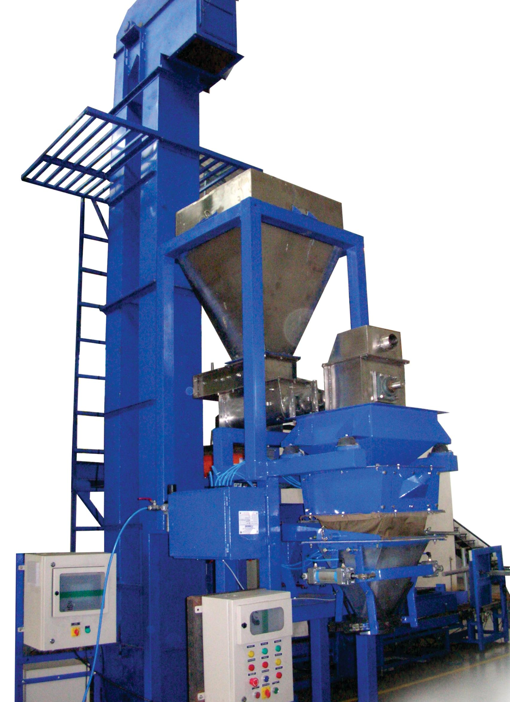
Complete Package with Raw Material Transfer to Packing Buffer Storage Specially Designed for Hazardous/food grade
