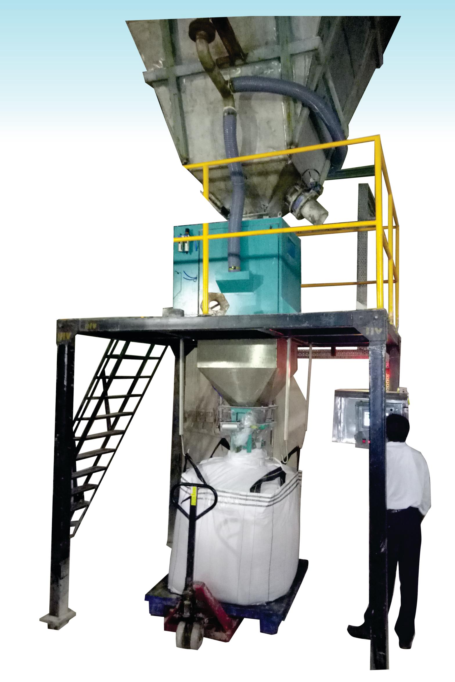
With Bag Inflation, Dust Collection Data Logging to PC/PLC/SCADA
